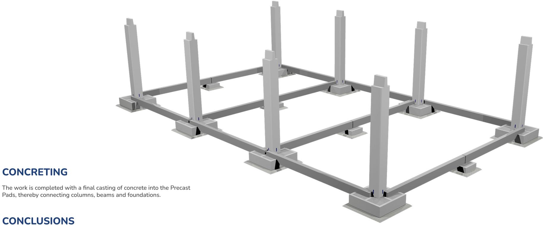
The use of the **Precast Foundation** eliminates all those inconveniences that crop up during the construction of foundations using traditional methods (for example, cast-in-place), aiming to halve the costs involved in constructing a foundation structure, greater jobsite safety for workers and a turnaround speed without precedence.
